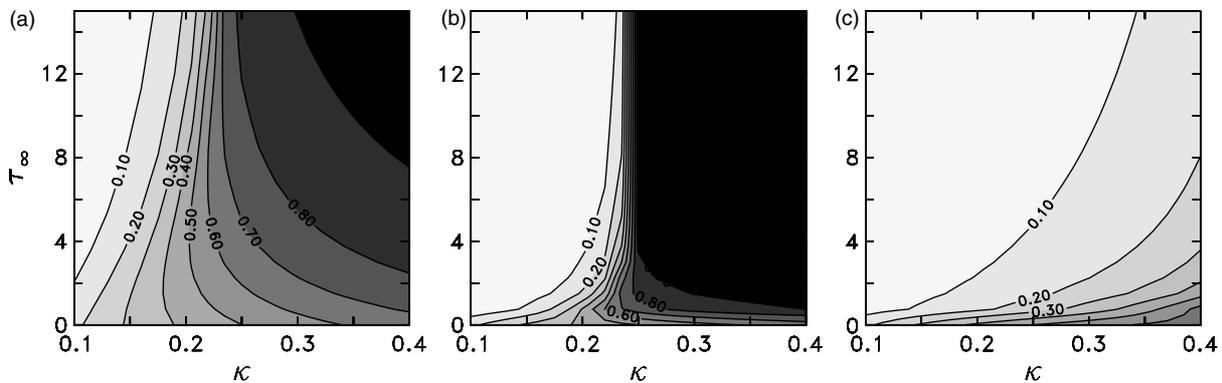
Figure 5. Adimensional tropopause level  $\eta_t$  as a function of  $\kappa$  and  $\tau_\infty$  assuming (a)  $\beta = 1$  and no pressure broadening, (b)  $\beta = 0.1$  and no pressure broadening, (c)  $\beta = 0.1$  and strong pressure broadening.
